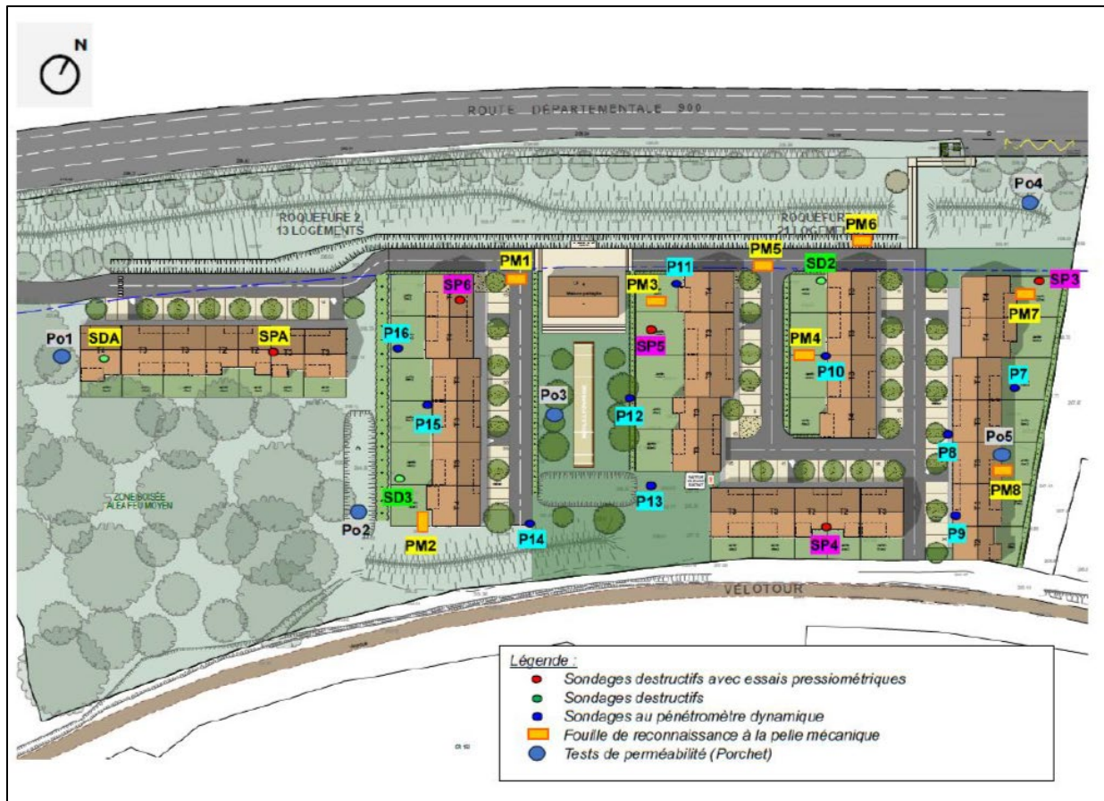
Figure 23: Implantation des sondages (source: GEOTECHNIQUE)
